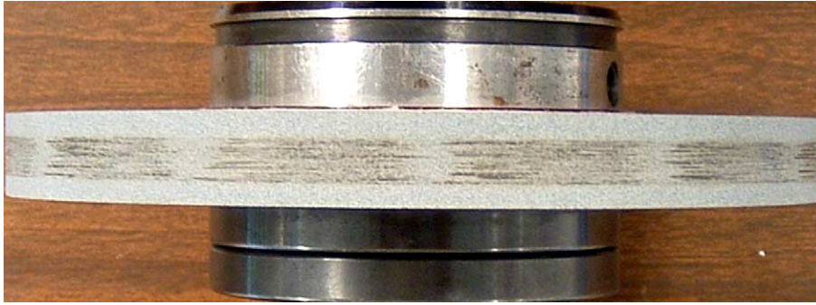
Fig. 5. The discoloration on the SiC wheel under high material removal rate (15 \mu\text{m} down feed and 4200 mm/min table speed) showing the intermittent nature of the marks and indicating repeated contact and separation of workpiece and wheel.
