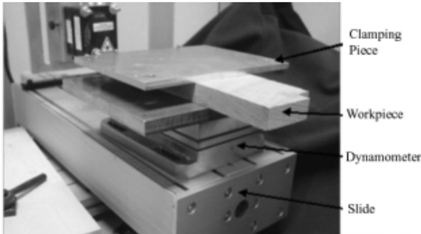
Figure 5. – Setup of the clamp, dynamometer, and slide for diamond wire cutting of wood.
